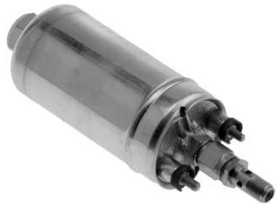
Bosch "044" 72.5 psi Fuel Pump, 200 LPH free flow.....Part No. FS FP044..... $259.99
